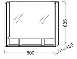
Product Specification: Mirror 80 cm - LH & RH lighting. EB1181. Collection: TERRACE. DIMENSIONS: 80 x 13 x 68.50 cm. WEIGHT: 14 kg. MATERIAL: Glass. INSTALLATION TYPE: Wall-mount. POWER: 230V, 14.4W, class II, IP 44. SHELF: Yes. TEMPERATURE: 4500°K. INSIDE STORAGE: Solid wood shelf. LED lighting left and right.
