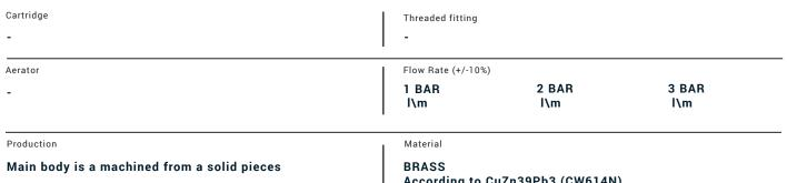
BRASS According to CuZn39Pb3 (CW614N) Max Lead content: 2.5%
