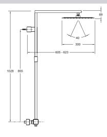
Product Specification: Shower column with thermostatic mixer. E98321. Collection: STRAYT. WEIGHT: 10 kg. MATERIAL: Metal. INSTALLATION TYPE: Wall-mount. WITH OR WITHOUT BRASSWARE: WITH TAPS AND FITTINGS. SHOWER TAPS-CLASSIFICATION: THERMOSTATIC.
