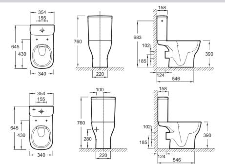
Product Specification: Rimless WC pan, P-trap. UJX101. Collection: STRUKTURA. DIMENSIONS: 64.50 x 34 cm. WEIGHT: 27 kg. MATERIAL: Ceramic. INSTALLATION TYPE: Floor-standing. NORMS AND REGULATION: NF. VOLUME OF WATER: 2.6/4 L and 3/6 L. HEIGHT: Standard. RIM TYPE: Rimless. RIM: Without rim. PRODUCT INCLUDED: (Cistern and seat not included). SEAT: Not included. TOILET BOWL FIXINGS: Concealed. Side inlet.
