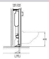
Product Specification: Floor support frame. E24155. Collection: NO COLLECTION. DIMENSIONS: 42 x 18 cm. WEIGHT: 17 kg. MATERIAL: 54. INSTALLATION TYPE: Self-supporting or install in front of a wall, inside a lightweight partition or inside a service duct. NORMS AND REGULATION: NF. VOLUME OF WATER: Standard 3/6 L. SINGLE/DUAL FLUSH: Dual flush. Supplied with wall fixings set (optional installation). Activation plate not included.
