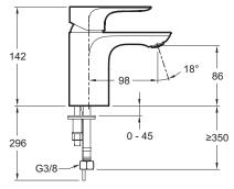
Product Specification: Single-lever washbasin lever with 5/35" system. E72277-4. Collection: ALEO. WEIGHT: 2 kg. MATERIAL: Metal. INSTALLATION TYPE: 1 hole. NORMS AND REGULATION: NF : I - ECAU : E00 Ch2 A3 U3 (Ps3) - ACS : 10 ACCLY 113. TYPE: Single-lever. FLOW RATE: 5 I/mn. HEIGHT UNDER SPOUT: 142. SPOUT PROJECTION: 98. CONNECTION: With supply hoses. MECHANISM: Cartouche à disques céramique. WASTE : Without waste. INSTALLATION TYPE: 1 hole. MECHANISM GUARANTEE: 5 years.
