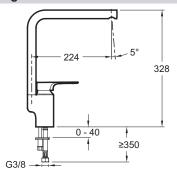
• MATERIAL: Metal • NORMS AND REGULATION: ACS: 11 ACC LY 540 • FLOW RATE: 10 I/mn • SPOUT PROJECTION: 224
