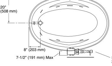
Pump/Control Access 20" (508 mm) W x 15" (381 mm) H
