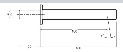
Product Specification: Wall-mount bath filler. E37344. Collection: STRAYT. WEIGHT: 1 kg. MATERIAL: Metal. INSTALLATION TYPE: Wall-mount. FLOW RATE: 30 I/min. SPOUT PROJECTION: 180.
