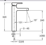
Product Specification: Tall single-lever washbasin mixer, smooth body. E98340. Collection: STRAYT. WEIGHT: 4.2 kg. MATERIAL: Metal. INSTALLATION TYPE: 1 hole. TYPE: Single-lever. FLOW RATE: 5 I/min. CONNECTION: With supply hoses. WASTE: Without waste. INSTALLATION TYPE: 1 hole. MECHANISM GUARANTEE: 5 years. No waste.
