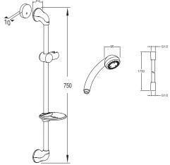
Product Specification: Shower and rod set. E14330. Collection: BASIC 2. WEIGHT: 1.3 kg. MATERIAL: Metal. INSTALLATION TYPE: Wall-mount.
