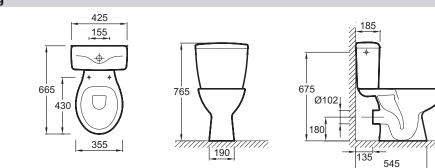
Product Specification: WC pack, P-trap. E0403. Collection: E0LIA. DIMENSIONS: 66.50 x 35.50 cm. WEIGHT: 36 kg. MATERIAL: Ceramic. INSTALLATION TYPE: Floor-standing. NORMS AND REGULATION: NF. VOLUME OF WATER: Standard 3/6 L. RIM TYPE: Open (traditional).
