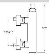
Product Specification: Single-lever wall shower mixer. E97368. Collection: AVID. WEIGHT: 3.5 kg. MATERIAL: Brass. INSTALLATION TYPE: 2 holes. TYPE: Single-lever. CONNECTION: With connectors and wall escutcheons. MECHANISM: Ceramic disc cartridge. INSTALLATION TYPE: 2 holes. MECHANISM GUARANTEE: 5 years. Non-return valve on shower outlet.
