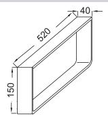
Product Specification: Towel rail bracket. EB507. Collection: PARALLEL. DIMENSIONS: 52 x 4 x 15 cm. WEIGHT: 1 kg. MATERIAL: Metal. INSTALLATION TYPE: Wall-hung. IMPORTANT: Towel rail bracket sold individually. Brushed metal.
