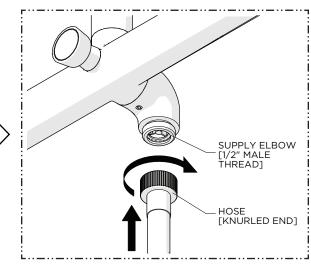
Thread the KNURLED END of the HOSE to the SUPPLY ELBOW on the VALVE BODY.
