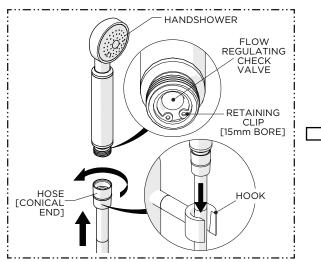
Thread the conical end of the HOSE to the HANDSHOWER then rest the HANDSHOWER on the HOOK.
