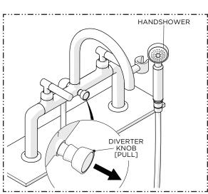
11. With water running, operate the DIVERTER KNOB to ensure it and the HANDSHOWER function properly then turn off the water.
