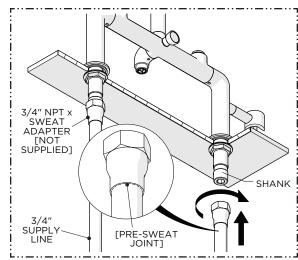
Pre-sweat 3/4" female NPT x sweat adapters to 3/4" supply lines and let cool. Apply a thin coat of pipe thread sealant to the male threads on the SHANKS then thread and securely tighten the ADAPTERS onto the SHANKS.
