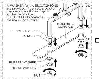
Insert the SHANKS into the holes on the mounting surface then attach the RUBBER and METAL WASHERS and NUTS onto the SHANKS. Securely tighten the NUTS against the underside of the mounting surface.
