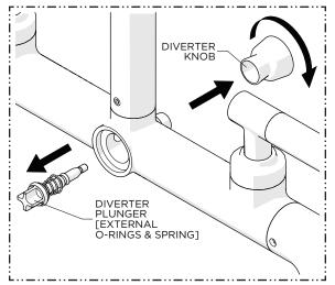
3. While holding the DIVERTER PLUNGER, unthread the KNOB from the PLUNGER then remove both parts.
