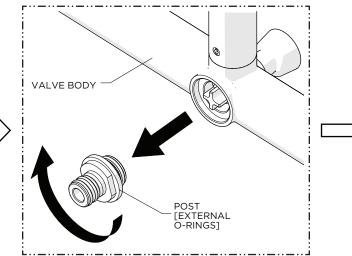
2. Unthread and remove the POST from the VALVE BODY.
