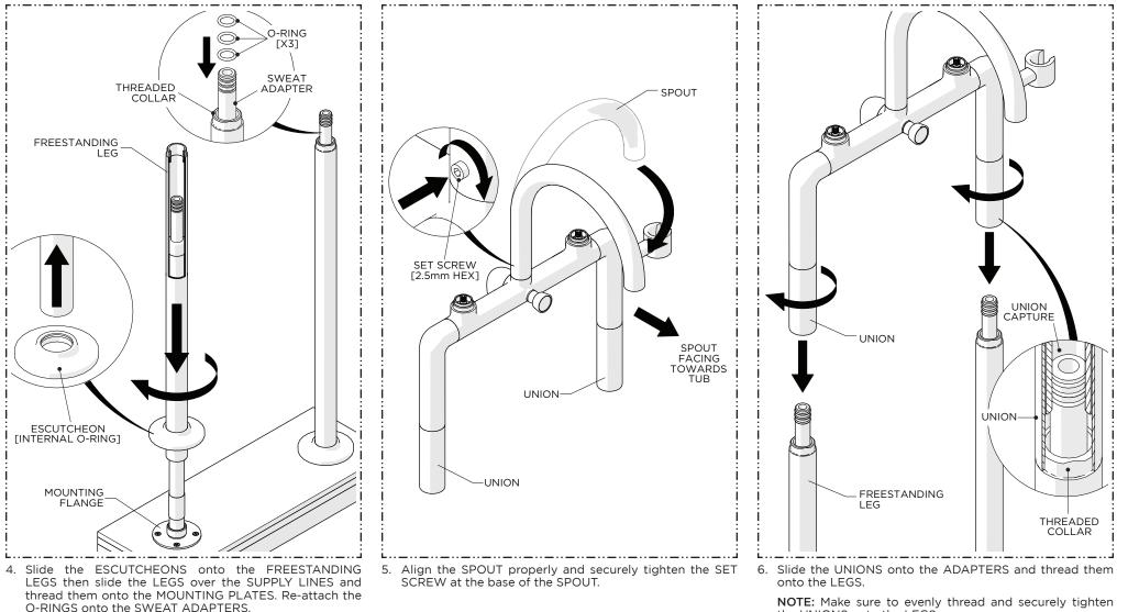
NOTE: Ensure the O-RINGS are not damaged and properly greased.
