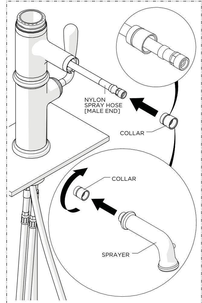
9. Unthread and remove the COLLAR from the SPRAYER inlet then slide the COLLAR over the SPRAY HOSE.
