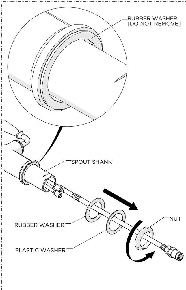
1. Unthread and remove the NUT from the SPOUT SHANK then remove the PLASTIC and RUBBER WASHERS.
