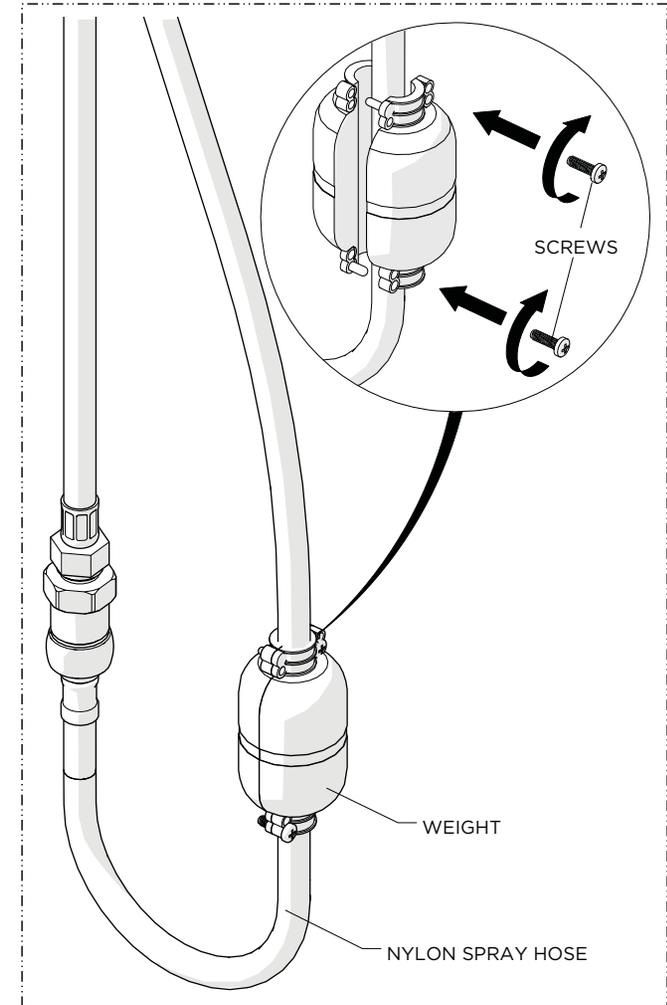
12. Align and press the two halves of the WEIGHT over the SPRAY HOSE in the desired position then thread and securely tighten the SCREWS provided.
