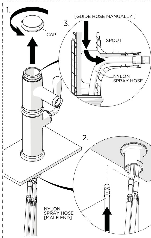
5. Unthread and remove the CAP from the top of the SPOUT then insert the MALE END of the NYLON SPRAY HOSE through the bottom of the SPOUT and, from above, manually guide the HOSE out of the SPOUT.
