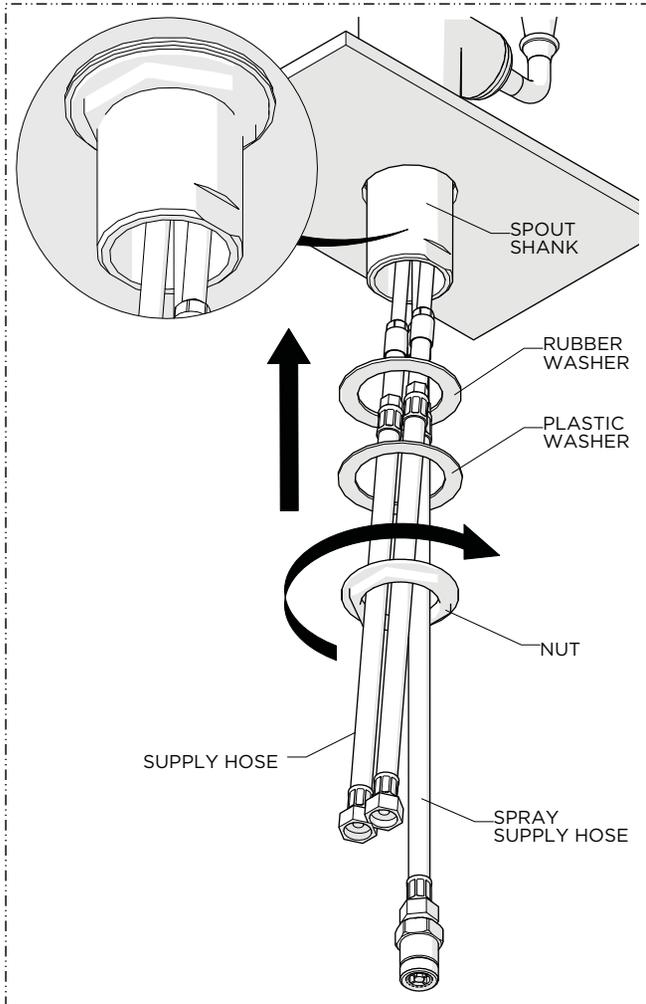
4. Slide the WASHERS and NUT over the HOSES then thread and securely tighten the NUT onto the SPOUT SHANK.
