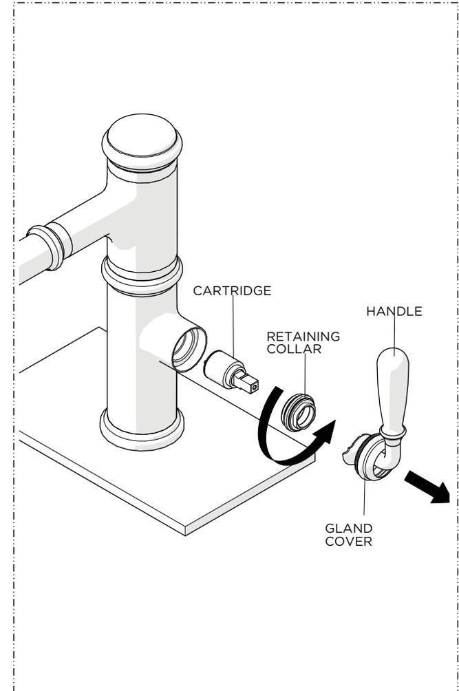
2. Remove the HANDLE then unthread and remove the RETAINING COLLAR to exposed and remove the CARTRIDGE.
