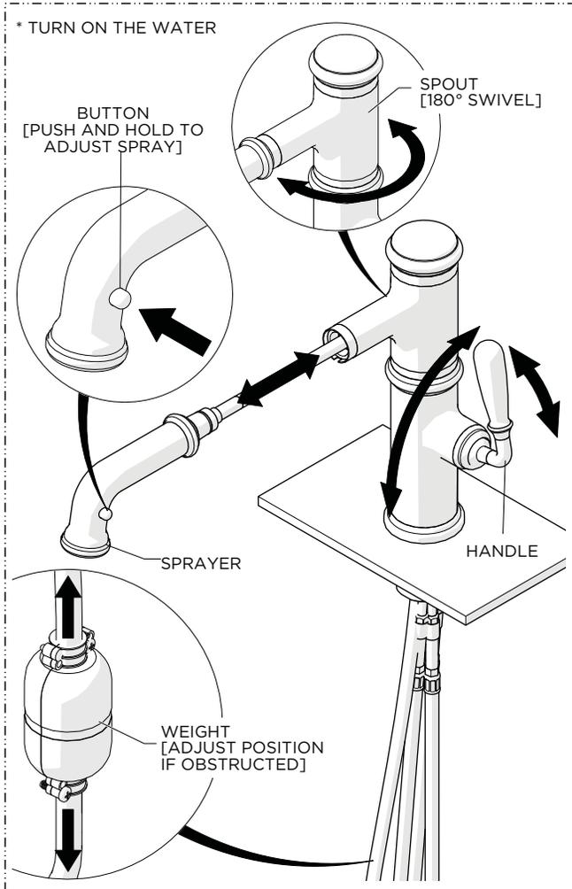
13. Turn on the water and operate the SPRAYER to ensure it functions properly making sure the WEIGHT can move freely beneath the cabinet and the SPOUT is able to swivel properly. Adjust the position of the WEIGHT if necessary.
