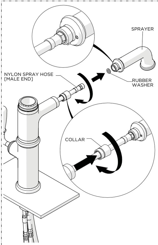
10. Thread and securely tighten the SPRAY HOSE into the SPRAYER using the RUBBER WASHER provided then thread and securely tighten the COLLAR back onto the SPRAYER.
