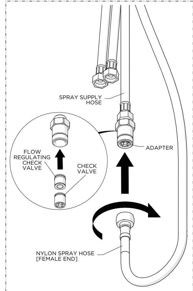
6. Thread and securely tighten the FEMALE END of the NYLON SPRAY HOSE onto SPRAY SUPPLY HOSE using the ADAPTER provided.
