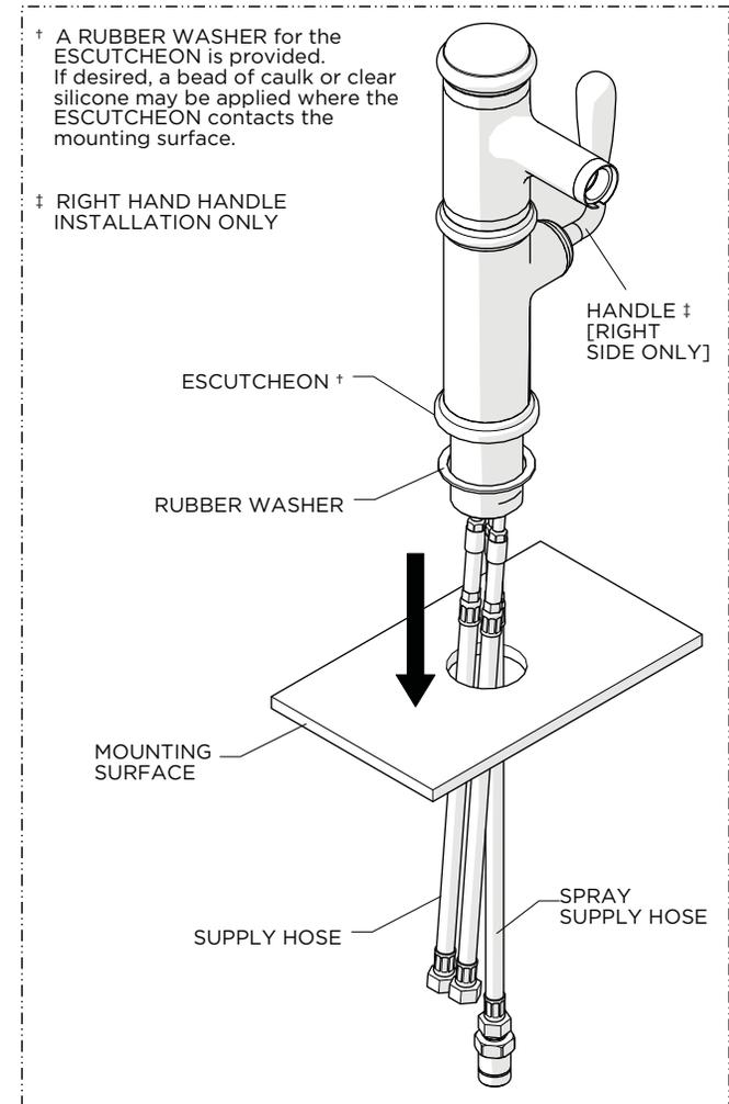
† A RUBBER WASHER for the ESCUTCHEON is provided. If desired, a bead of caulk or clear silicone may be applied where the ESCUTCHEON contacts the mounting surface.
