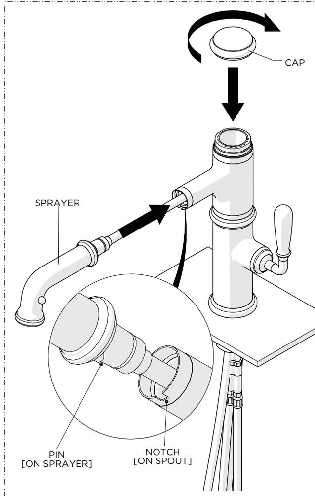
11. Insert the SPRAYER into the SPOUT then thread the CAP back onto the top of the SPOUT.
