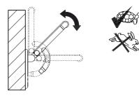
Check friction on both sides of the seat.
