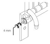
Clockwise: increase braking force Counter-clockwise: reduce braking force
