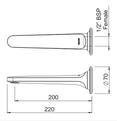
CONSTRUCTION: Eco Brass CLASSIFICATION: Suitable for all pressure systems INLET CONNECTIONS: 1/2 " BSP Female OUTLET CONNECTION: N/A WORKING PRESSURE: 35-1000kPa OPERATING TEMPERATURE: 5 °C - 80 °C
