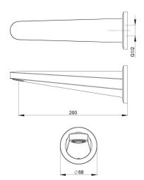
**CONSTRUCTION:** Brass body **PROJECTION:** 200mm
