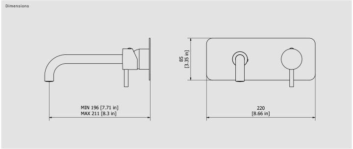
Cartridge Threaded fitting G1/2" female Ø35 ceramic cartridge Aerator Flow Rate (+/-10%) 1 BAR 2 BAR 3 BAR M16.5X1 7.6 l\m 10.5 l\m 13 I\m
