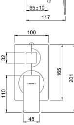
**CONSTRUCTION:** Eco Brass CARTRIDGE TYPE: Rotary Ceramic CLASSIFICATION: Suitable for mains pressure only **INLET CONNECTIONS:** 1/2 " BSP Female **OUTLET CONNECTIONS:** 1/2 " BSP Female WORKING PRESSURE: 150 - 1000kPa OPERATING TEMPERATURE: 5 °C - 80 °C
