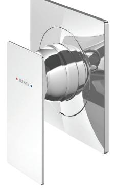
CONSTRUCTION: Brass body CARTRIDGE TYPE: Ceramic with Fastflow II technology CLASSIFICATION: Suitable for all pressure systems CONNECTIONS: 1/2 " BSP Male WORKING PRESSURE UNEQUAL COLD: 17 - 120kPa WORKING PRESSURE UNEQUAL HOT: 300 - 500kPa (If supply exceeds 500kPa a pressure limiting valve must be installed) DIMENSIONS FOR FITTING: Ø100mm hole OPERATING TEMPERATURE: 5 °C - 80 °C
