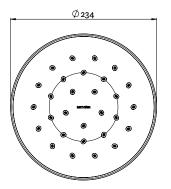
CONSTRUCTION: Brass adjustable ball joint connection CLASSIFICATION: Suitable for all pressure systems WORKING PRESSURE: 35 - 500kPa DIMENSIONS FOR FITTING: 1/2" BSP OPERATING TEMPERATURE: 5 °C - 70 °C
