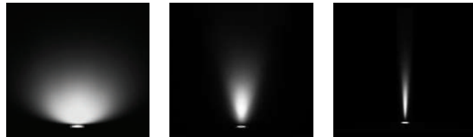
U-D 90° Ultra-wide Beam M 25° Medium Beam C 8° Narrow Beam
