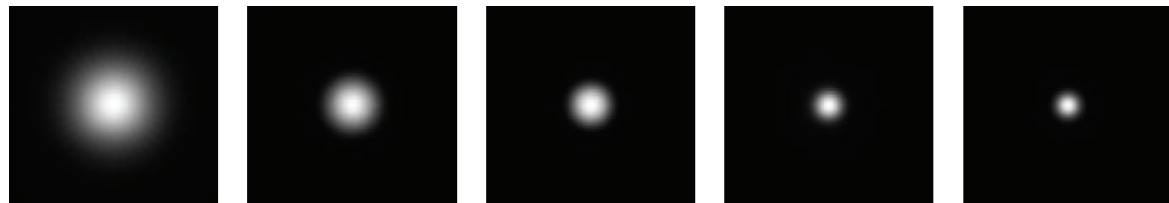
U-D 90° Ultra-wide Beam D 40° Wide Beam M 25° Medium Beam C 11° Narrow Beam U-C 6° Ultra-narrow Beam
